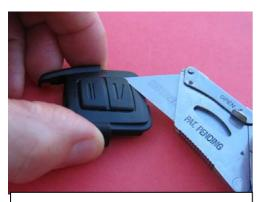
5. Old buttons are an over mould to the cover and have to be cut of with the sharp blade of scalpel, stanley knife or side-cutter
