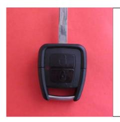
10. Close remote control and audibly latch into key part. Test buttons as your remote works straight away with no need for reprogramming.
